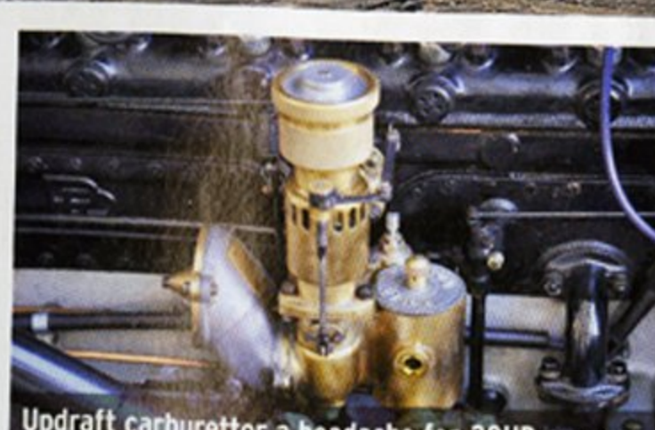
Updraft carburettor a headache for 20HP owners.
